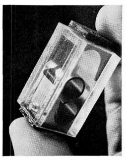
TYPICAL ROLAMITE configuration is used here as a gravity switch. The cutout in the band around the rollers helps introduce a force into the roller cluster equal to a specified gravity, such as 12 G's. When an accelerating vehicle reaches this G-level, the cluster breaks away, snaps to the right, and closes (or opens) an electrical circuit.
